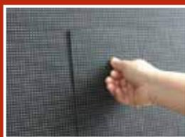
A handle facilitates the dismantling of the pixel card.
