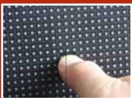
By pushing the marked point the module comes out.
