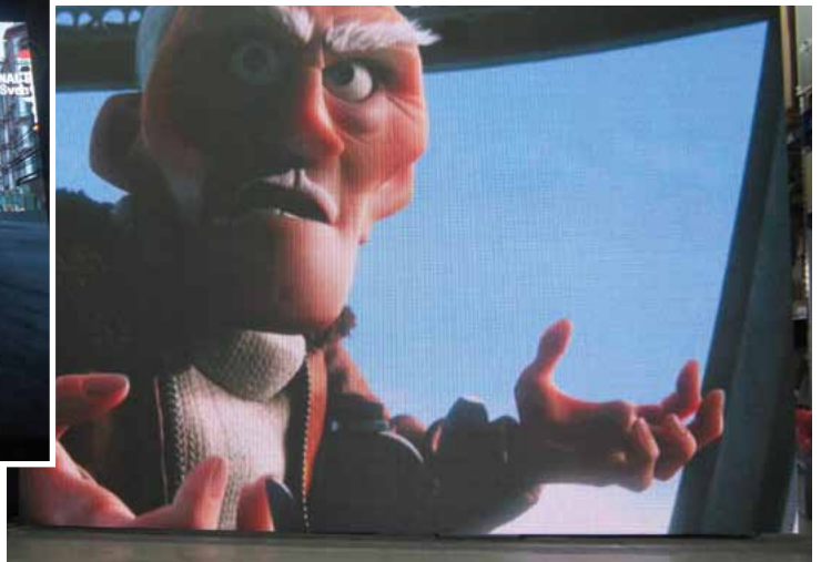
L - 9 SI display 4.6 x 3.4 m | 8 x 6 module, 9 mm pixel pitch
