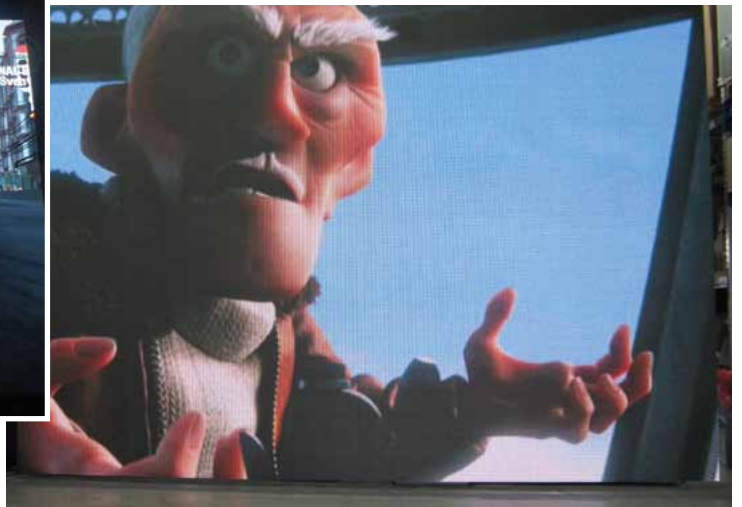
L - 9 SI Display 4.6 x 3.4 m | 8 x 6 Module, 9 mm Pixelabstand
